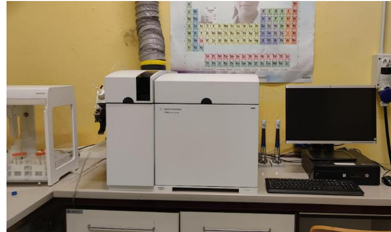
Inductively Coupled Plasma Mass Spectrometry (ICP-MS)
